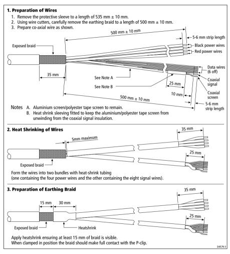
7. Fit the 8-way plug (supplied in the kit of parts) to the cable as shown in the following diagram. The terminal clamps are operated using a screwdriver as shown.
